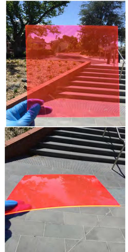
Laboratory samples of thin LSC Perspex with no PV cell
